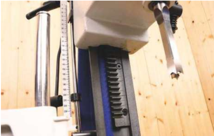
▲ The rack and pinion slide on the plunge head keeps things running smoothly
